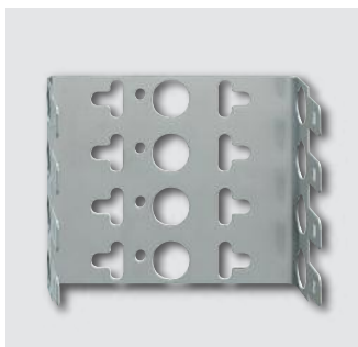
MB 4 221 004 ● Mounting bar for LSA-connection elements, 10 pairs, grid dimension 22.5 mm, for 4 modules, installation height: 22 mm, 104,5 x 87,5 x 42 mm, 98 g
