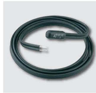
Temperature sensor 700 802 201 ● Resolution 1 °C, B-value 3435 K ± 1%, 10 kΩ at 25 °C, black (similar RAL 9005), 600 mm, 6 g
