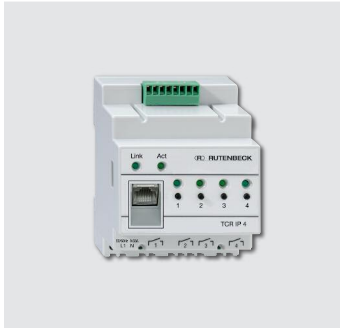
TCR IP 4 700 802 610 ● DIN-rail mounting housing 4 DIN units wide, light grey (similar RAL 7035), 72 x 90 x 65 mm, 298 g
