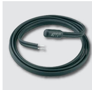
Temperature sensor 700 802 201 ● Resolution 1 °C, B-value 3435 K ± 1%, 10 kΩ at 25 °C, black [similar RAL 9005], 600 mm, 6 g
